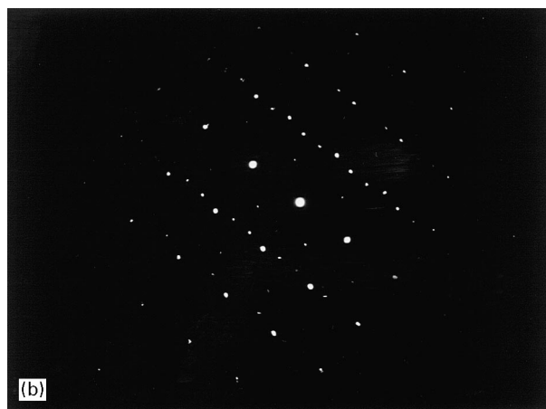
Figure 7 SAD patterns illustrating the formation of a Nishiyama-Wasserman type orientation relationship between the \gamma' and \beta -phases in the intradendritic region of the Ni-26 at % Al-21 at % Cr-11 at % Ti material held for 140 h at 850 °C. (a) B = [\bar{1}01]_{\gamma'} , (b) B = [001]_{\beta} \parallel [\bar{1}01]_{\gamma'} .
