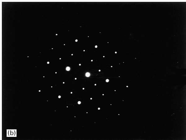
Figure 2 Microstructure of the β'-α eutectic mixture. (a) BF micrograph showing the as-cast Ni-25 at % Al-20 at % Cr-15 at % Ti alloy (c, β', d, α). (b) SAD pattern with B = [110]_{\alpha,\beta'} showing the cube-cube orientation relationship of the eutectic β' and α phases (Ni-25 at % Al-24 at % Cr-15 at % Ti alloy aged for 140 h at 850 °C).
